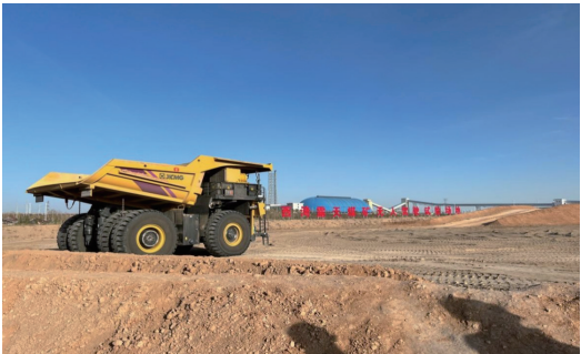
▲ Figure 240-ton heavy-duty hybrid mining truck
